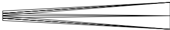
Light path of a 6" refracting telescope, which is expanded to f/30 with a Barlow lens (light coming from the left).
