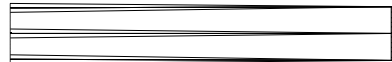
Light path of a 6" refracting telescope, which is expanded to f/30 with a telecentric system (light coming from the left).
